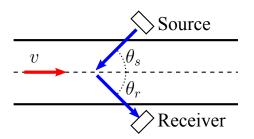
With  $\theta_r = \theta_s = 30^\circ$ , the doctor detects a frequency shift of 1200 Hz. Assume that the speed of sound in blood is 1500 m/s and the vessel cross-sectional area is 2 cm<sup>2</sup>. What is the patient's volumetric flow rate through the vessel?
