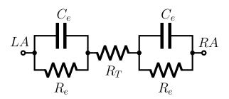
Here,  $R_e$  and  $C_e$  represent the double-layer formed in the gel electrodes and  $R_T$  represents the impedance of the thoracic cavity.  $R_T$  changes as the person breathes, which can be measured.
