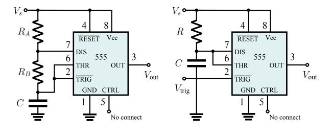
$T_{\rm hi} = 0.7(R_A + R_B)C$   $T_{\rm lo} = 0.7R_BC$  T = 1.1RC
