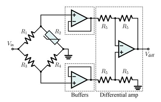
(a) [2 pts] Assume the op-amps are ideal. Write an expression for  $V_{\text{diff}}$  in terms of the resistances and  $V_{\text{in}}$ . *Hint:* What is the differential gain of the differential amplifier?
