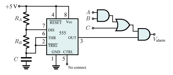
The digital outputs of three different medical instruments are connected to the inputs A, B, and C. Under certain conditions, the circuit outputs a square wave which drives an alarm speaker. This alerts medical staff of an emergency.
