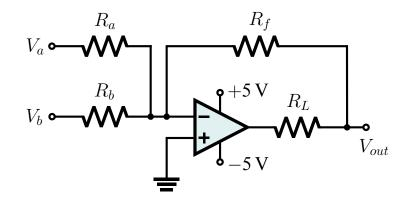
(a) Assume the operational amplifier is ideal and unsaturated. Derive from first principles an expression for  $V_{out}$  in terms of  $V_a$  and  $V_b$ .
