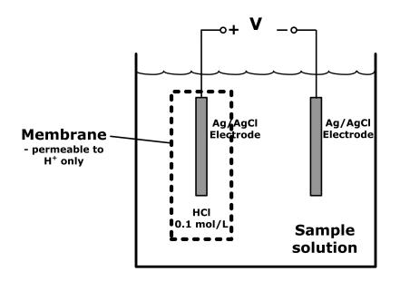
The Nernst potential equation for ion A<sup>n</sup> where n is valance of the ion:
