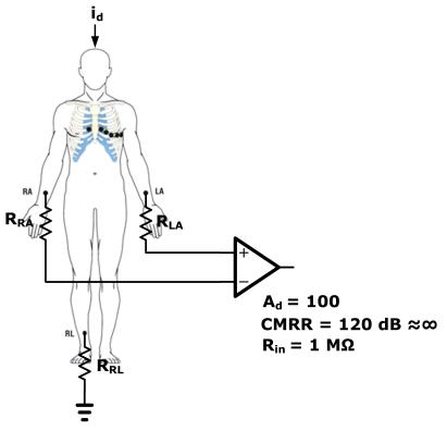
a. [15 pts] Find the differential gain  $A_{d1}$ , common-mode gain  $A_{c1}$  and CMRR<sub>1</sub> of the overall system with the bioinstrumentation amplifier connected to the RA and LA electrodes on the body.
