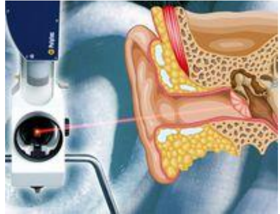
A laser Doppler vibrometer (Polytec) interrogating the eardrum
