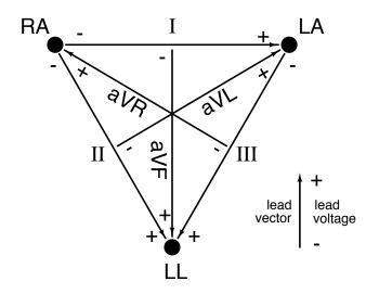
(a) [8 pts] You are given an instrument that outputs the six-lead frontal ECG. However, four of the leads are malfunctioning, and only leads I and aVF provide useful outputs. Reconstruct the missing leads of the frontal ECG from the lead I and lead aVF outputs:
