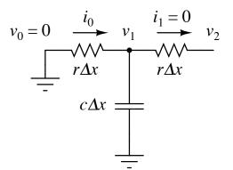
1. (10 points): Write the ordinary differential equation governing the dynamics of the voltage  $v_1(t)$  at the center of the cable. What can you say about the voltage  $v_2(t)$  on the right end?
