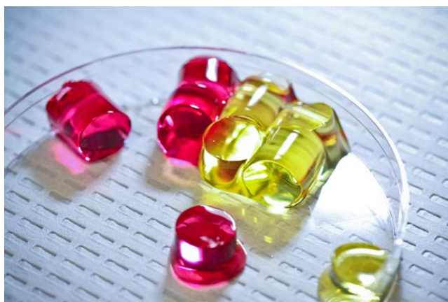
Figure 1. Various forms of hydrogel base on the materials that are mixed with water [3].
