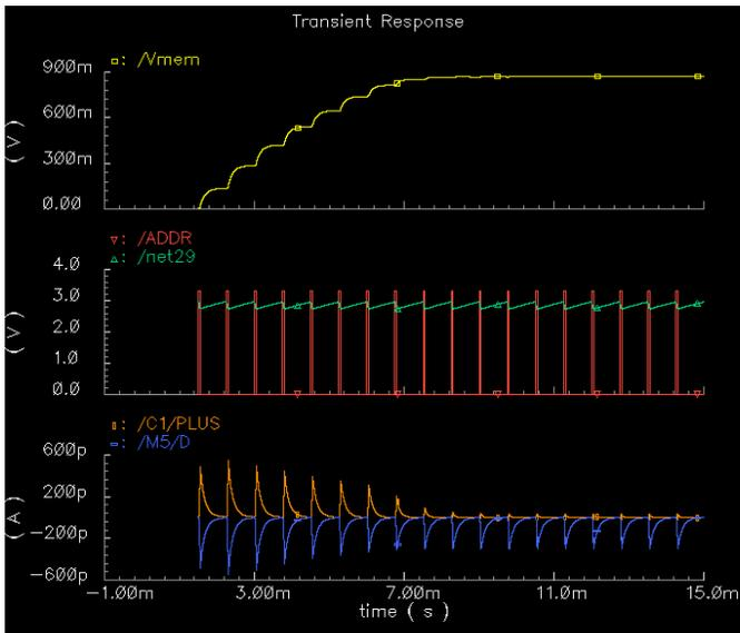
Fig. 5. Simulation results for the synapse. The top trace is the membrane potential. The second trace overlays incoming action event pulses with the voltage on  $C_{syn}$ . The bottom trace shows the current through  $M6$  (positive going) and the current onto the membrane capacitance (bottom going).
