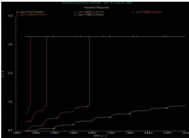
Fig. 6. Membrane voltage for different spike input frequencies.
