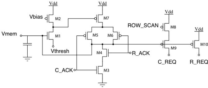
Fig. 2. Integrate and Fire Neuron [3] Schematic
