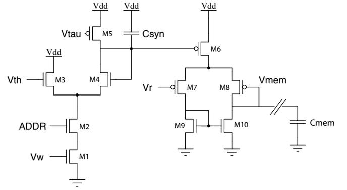
Fig. 3. Conductance Based Synapse Schematic.  $V_{mem}$  and  $C_{mem}$  are shared with the neuron.
