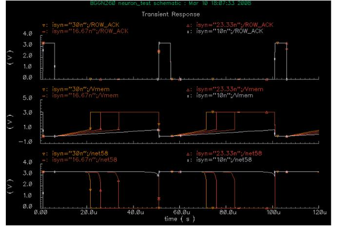
Fig. 4. Simulation results for the neuron. The top trace is the external reset signal, the middle trace the membrane voltage, and the bottom trace is the output of the common source amplifier.
