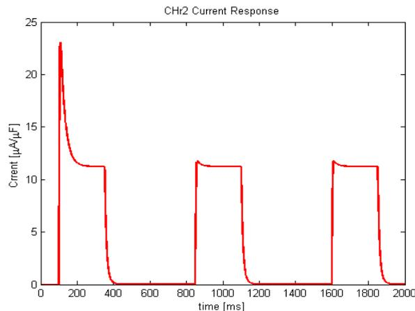
Figure 4:ChR2 current response after stimulation with 2.5 mW, 470 nm light source lasting 300ms per pulse
