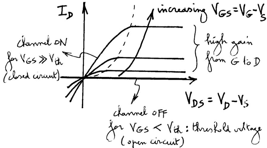
Simple model of channel conductance  $g_{ds} = \frac{\partial I_D}{\partial V_{DS}}$ :
