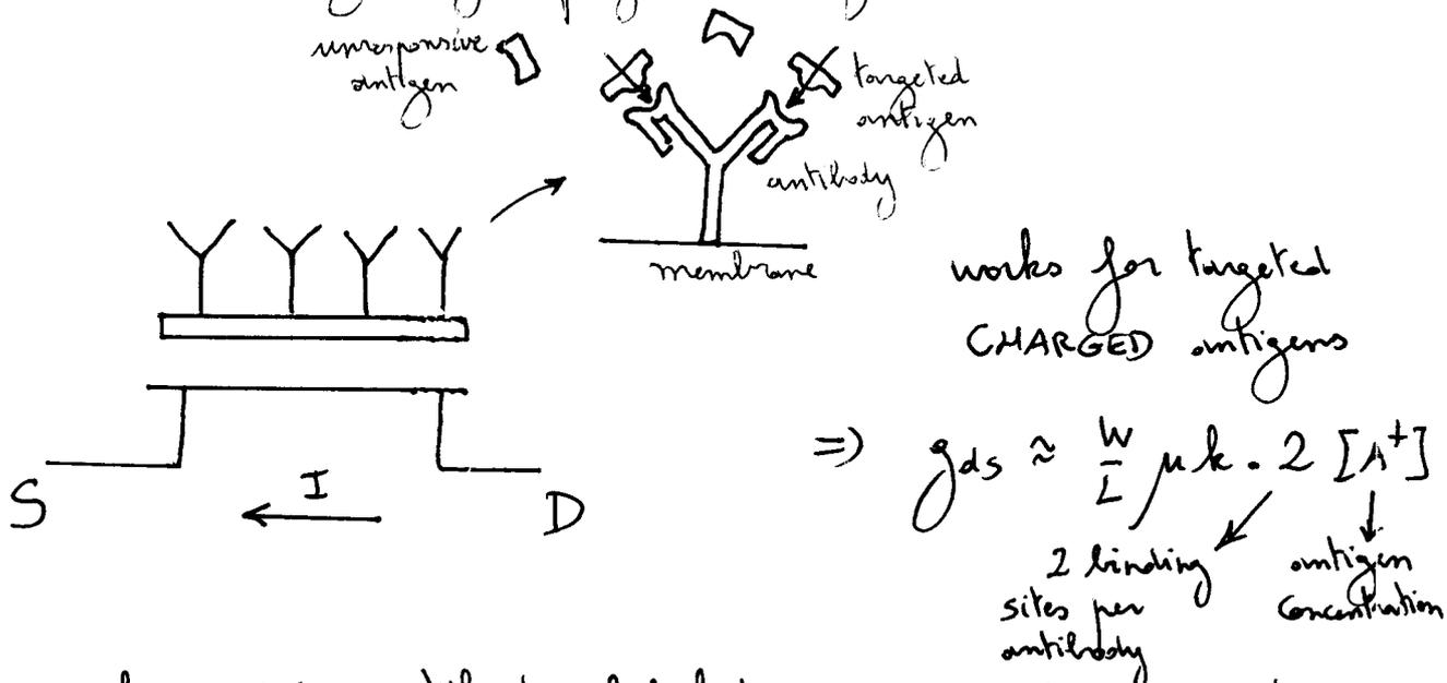
Arrays of various antibody labeled IMFETS integrated with MOSTFET amplification and selection circuits allow for high-throughput pathogen detection on a single microchip.
