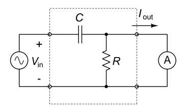
(a) [10 pts] Find the input impedance  $Z_{in}(j\omega)$ .
