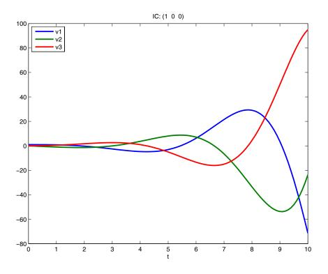
Figure 6: Ring oscillator ODE solution for  $\mathbf{v}(0) = (1,0,0)^T$ .
