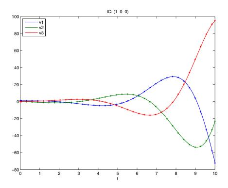
Figure 10: Ring oscillator ODE simulation using the Matlab built-in ode23 numeric ODE solver.
