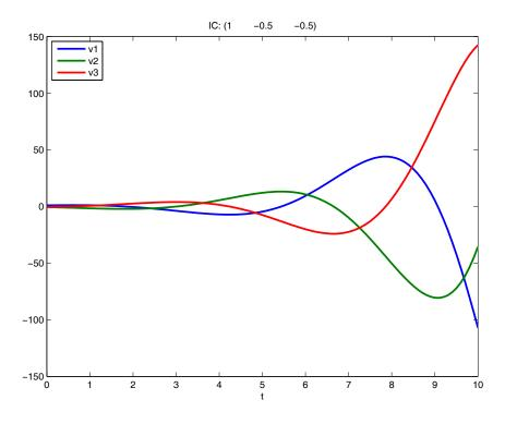
Figure 5: Ring oscillator ODE solution for  $\mathbf{v}(0) = (1, -\frac{1}{2}, -\frac{1}{2})^T$ .
