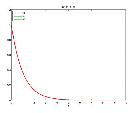
Figure 4: Ring oscillator ODE solution for  $\mathbf{v}(0) = (1, 1, 1)^T$ .
