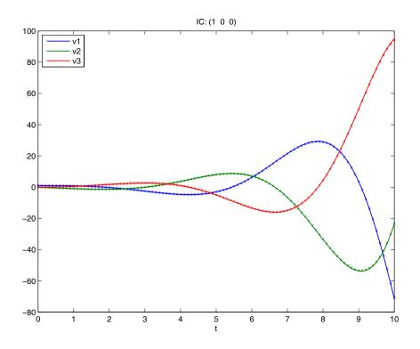
Figure 8: Ring oscillator ODE simulation using Crank-Nicolson integration.
