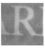
Fig. 9. Example image acquired from the adaptive imager chip after gain mismatch reduction. We projected a light-grey letter "R" against a dark-grey background onto the chip.
