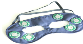
Fig. 3. Bio-cursor head-mask with six EOG electrodes.
