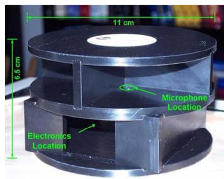
Fig. 1. Acoustic enclosure (ASU) with microphones and electronics.
