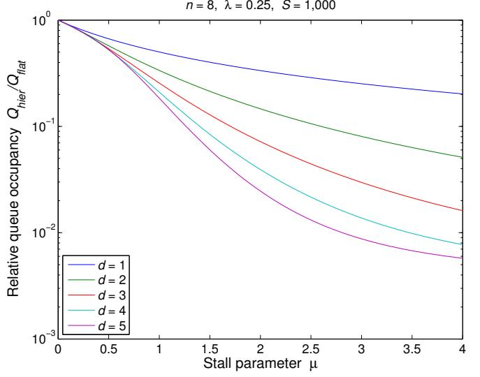
Fig. 6. Queue occupancy in hierarchical routing  $Q_{hier}$  relative to flat synaptic routing  $Q_{flat}$ , as a function of geometric stall factor  $\mu$ .
