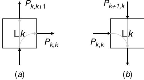
Fig. 3. Probabilistic model of event routing at level  $k$  in the routing hierarchy. (a): Event messages from children are routed to siblings and the parent. (b): Event messages from parents or siblings are routed only to children.
