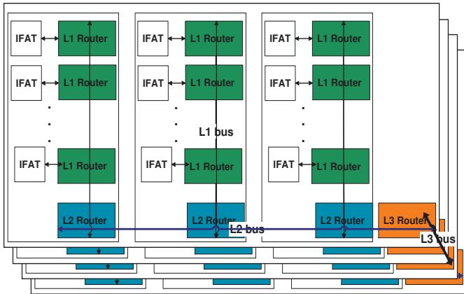
Fig. 1. Multi-chip hierarchical spike event communication architecture, with integrate-and-fire array transceiver (IFAT) neuronal blocks, and multi-level neural event routers
