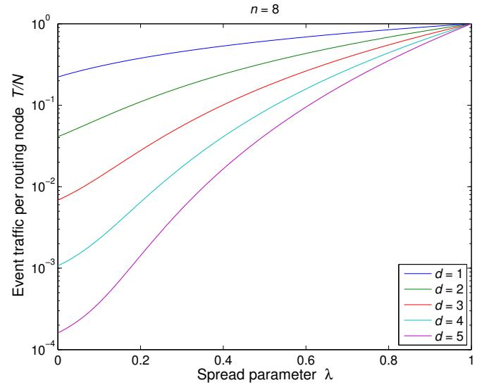
Fig. 5. Traffic overhead  $T/N$ , as the number of global messages per spike event per routing node, as a function of geometric spread factor  $\lambda$ .
