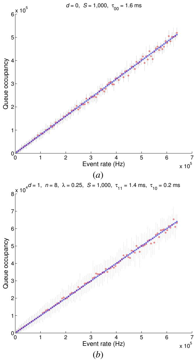
Fig. 7. Observed random, average, and theoretical queue occupancy as a function of event rate, (a) for a flat hierarchy with delay  $\tau_0 = 1.6 \text{ ms}$ , and (b) for a depth  $d = 1$  hierarchy with  $\lambda = 0.25$ ,  $n = 8$ ,  $\tau_{11} = 1.4 \text{ ms}$ , and  $\tau_{10} = 0.2 \text{ ms}$ . Global synaptic fan-out  $S = 1,000$  in both cases.
