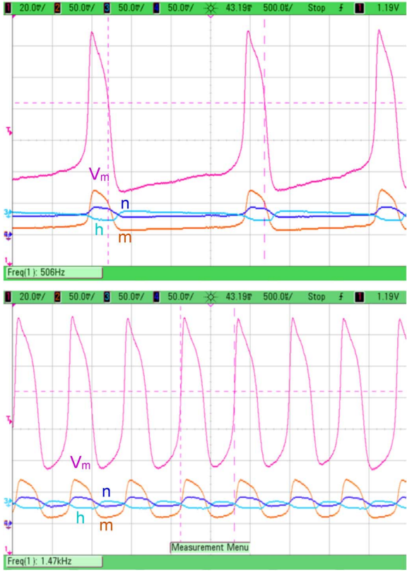
Fig. 12. Measured dynamics of membrane voltage V_m and gating variables n , m , and h for a single HH neuron. (a) and (b) show the effect of setting the global temporal scale parameter I_\tau , uniformly speeding or slowing the dynamics across all variables.
