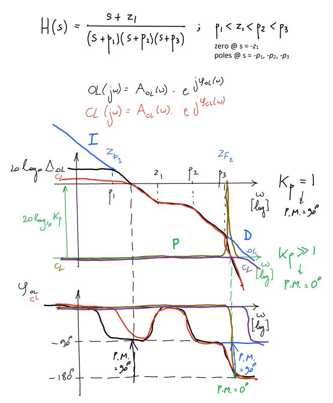
Bode design of proportional-integral-derivative (PID) control:
