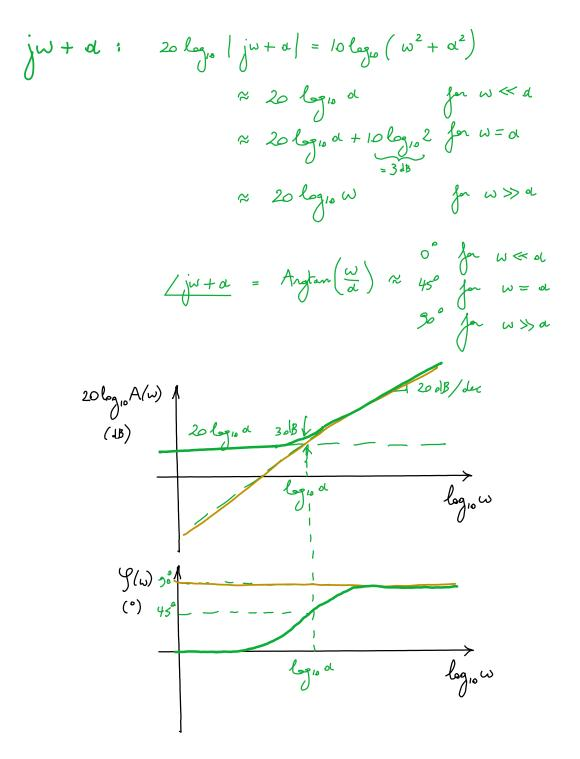
To first order, each **zero** (@ s = -a) contributes a **20 dB/dec rise in slope** of log amplitude, and a **+90° step** in phase, for radial frequencies **above** the magnitude of that zero ( $\omega > |a|$ ).
