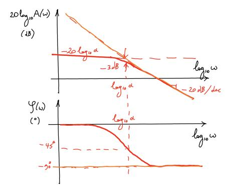
To first order, each **pole** (@ s = -a) contributes a -**20 dB/dec decline in slope** of log amplitude, and a -**90° step** down in phase, for radial frequencies **above** the magnitude of that zero ( $\omega > |a|$ ).
