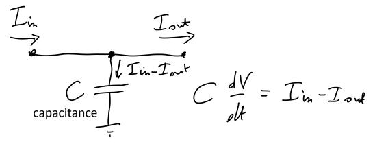
Resistance and capacitance/compliance combined (lumped electrical model):
