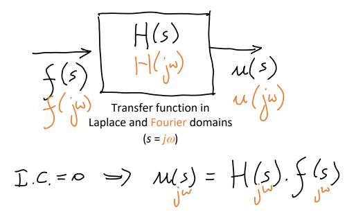
For zero initial conditions (I.C.), the system response u to an input f is directly proportional to the input.
