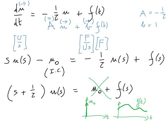
A non-zero I.C.  $u(0) = u_0$  is equivalent to an additional driving force  $f(t) = u_0 \delta(t)$ .
