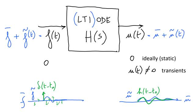
A system is *stable* when small-signal perturbations give rise to *bounded* transients over time in the system response.
