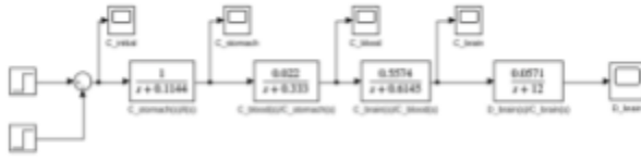
Figure 2. Transfer function block diagram of the system
