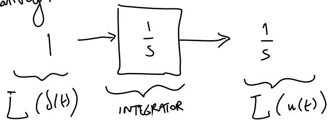
The time integral of the impulse response of a LTI system is the step response of that LTI system.
