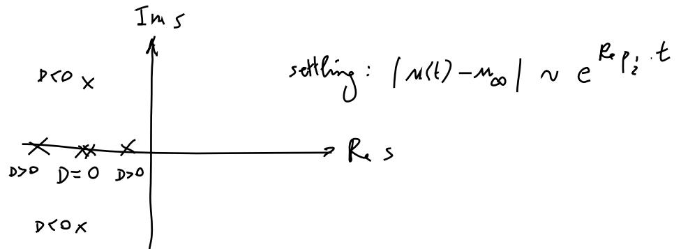
$$D = \gamma^2 - 4Km = 0 \quad \Rightarrow \quad K = \frac{\gamma^2}{4m}$$
