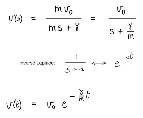
The velocity v decays exponentially, from its initial value, at a rate given by damping over mass.
