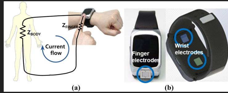
(a) Directional loop of current of device and body
