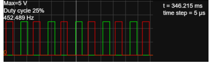
Fig. 13. V_{Red} (red) and V_{IR} (green) of the Alternating LED Activator with 5V power supply.
