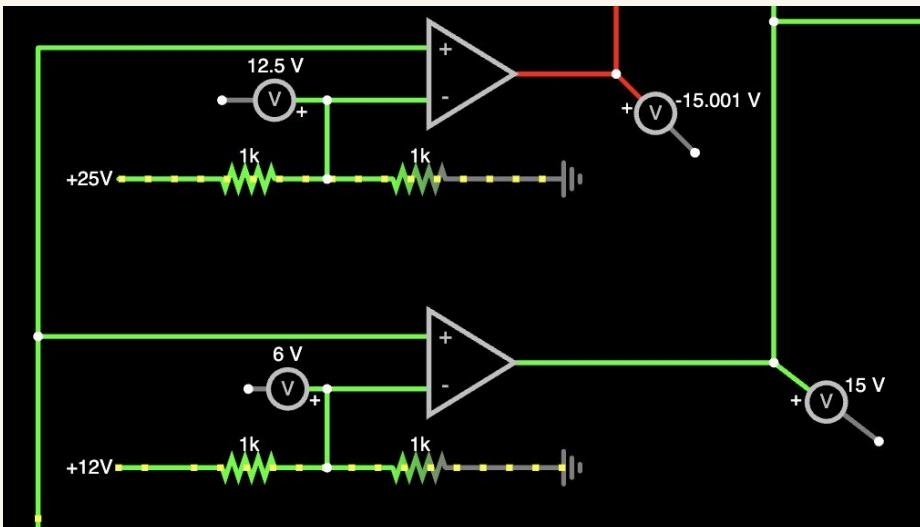
Compares the magnitudes of two voltages ( $V_{in}$  and  $V_{ref}$ ) and determines which is the largest of the two
