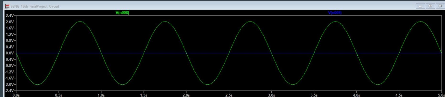
Blue - Input sine wave:  $V_{pp} = 0.002V @ 1Hz$
