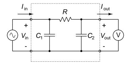
(a) [10 pts] Find the input impedance  $Z_{in}(j\omega)$ .
