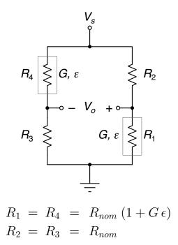
(a) [10 pts] Find the output voltage  $V_o$  as a function of stress  $\sigma$ . Is the response linear, and why?
