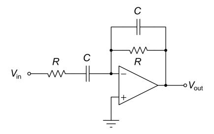
(a) [15 pts] Assume the operational amplifier is ideal and unsaturated. Derive the transfer function  $H(j\omega) = V_{out}(j\omega) / V_{in}(j\omega)$ . What type of filter is this? Identify the poles and zeros, and the frequency at which the transfer function  $H(j\omega)$  reaches its peak magnitude. (b) [5 pts] What is the input impedance at the  $V_{in}$  node?
