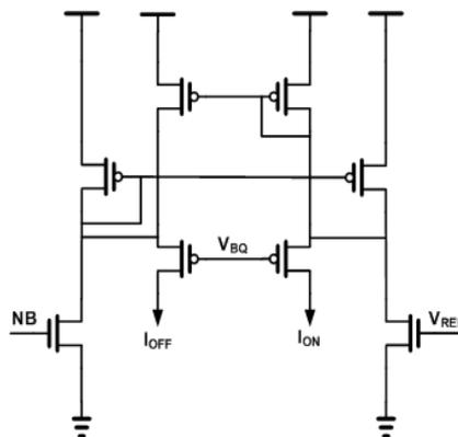
Figure 4: Circuit schematic of on and off bipolar cells
