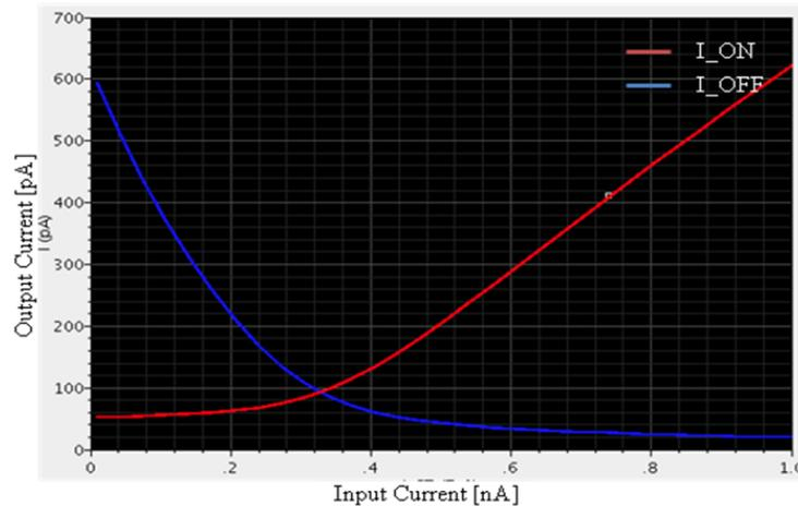
Figure 7: Simulation results of on and off currents versus input current to the bipolar circuit
