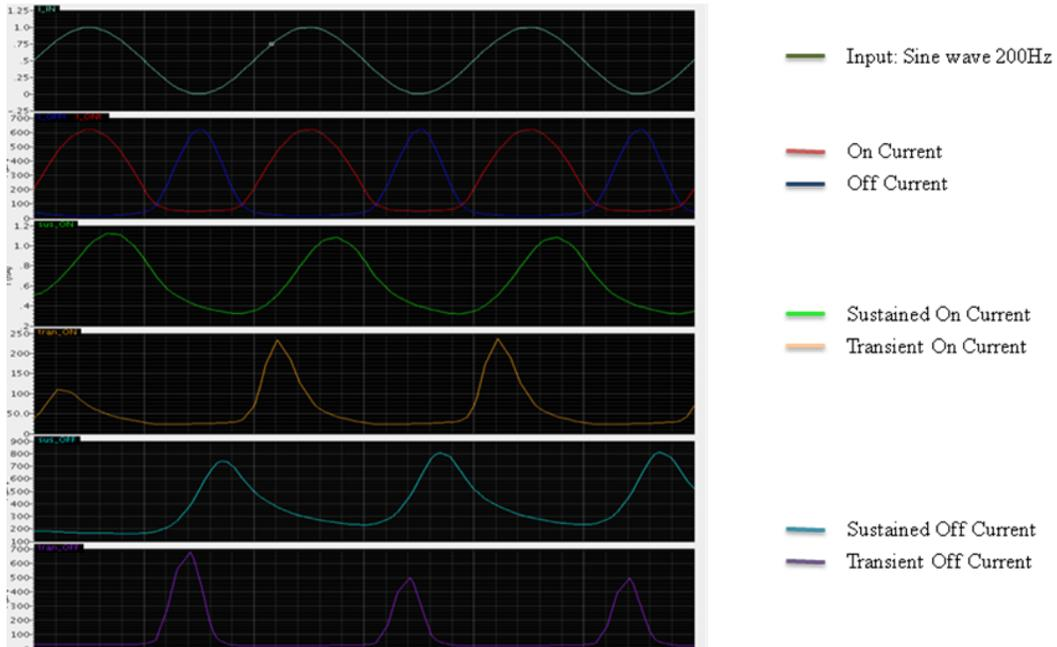
Figure 9: On/off sustained and transient responses from 200Hz sin wave input
