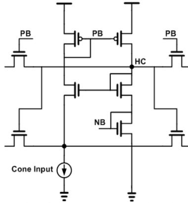
Figure 2: Circuit schematic of the cone terminal and the horizontal cell (HC)
