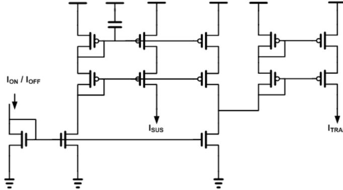
Figure 5: Circuit schematic of sustained and transient pathways to ganglion cells
