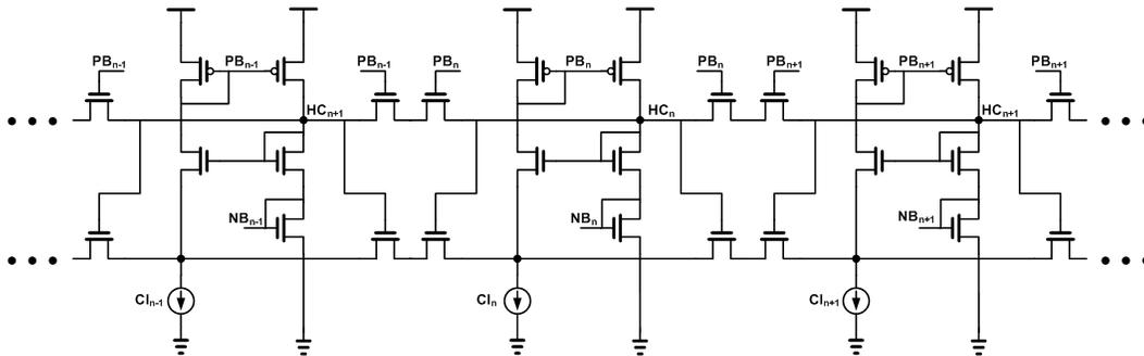
Figure 3: One-dimensional structure of cone terminals and horizontal cells
