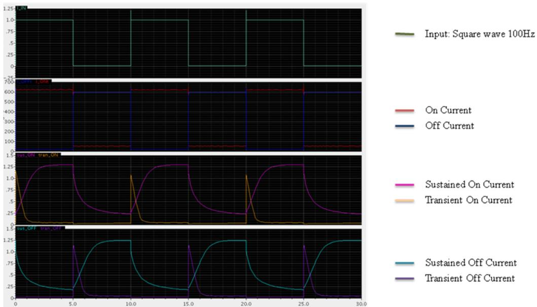
Figure 8: On/off sustained and transient responses from 100Hz square wave input
