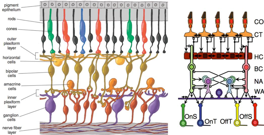
Figure 1: Simple anatomy of the retina [19] (left) and its corresponding structure of the silicon retina [17] (right). CO stands for cone, CT for cone terminal, HC for horizontal cell, BC for bipolar cell, NA for narrow-field amacrine cell and WA for wide-field amacrine cell. It also includes on/off sustained ganglion cells (OnS and OffS) and on/off transient ganglion cells (OnT and OffT).
