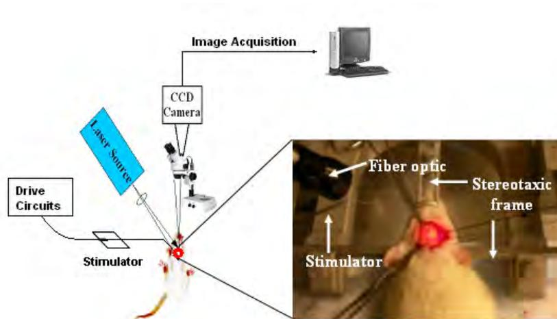
Laser speckle functional imaging of microvascular neural activity on cortical surface, through thinned skull.
