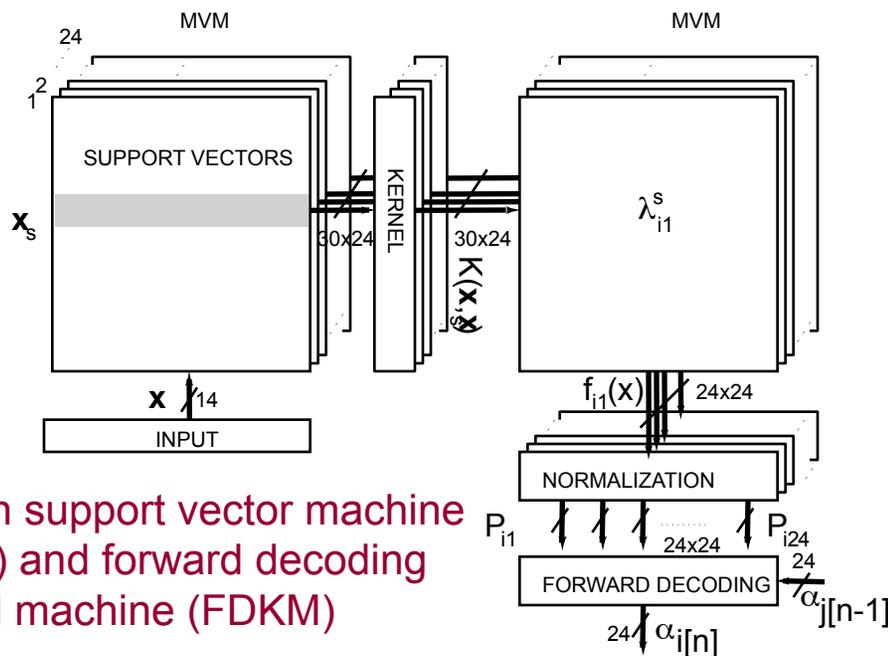
Silicon support vector machine (SVM) and forward decoding kernel machine (FDKM)
