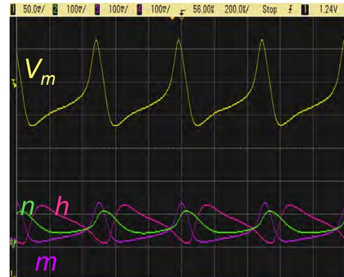
Recorded dynamics of action potential and channel kinetics for one HH neuron.
