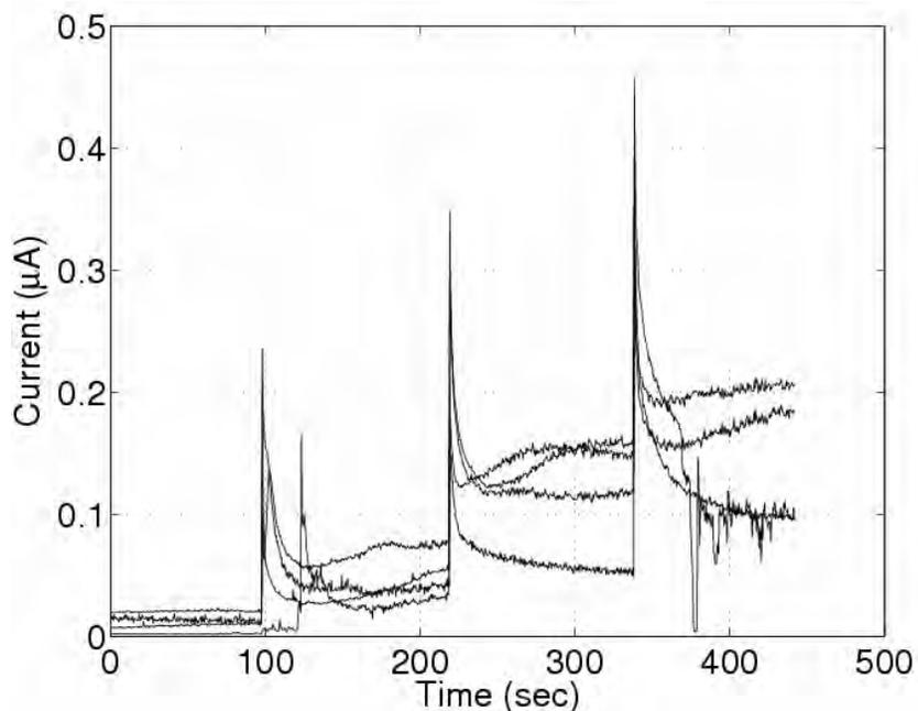
*"In vitro"* Dopamine monitoring by the chip using micro-fabricated electrode array as working electrode.
