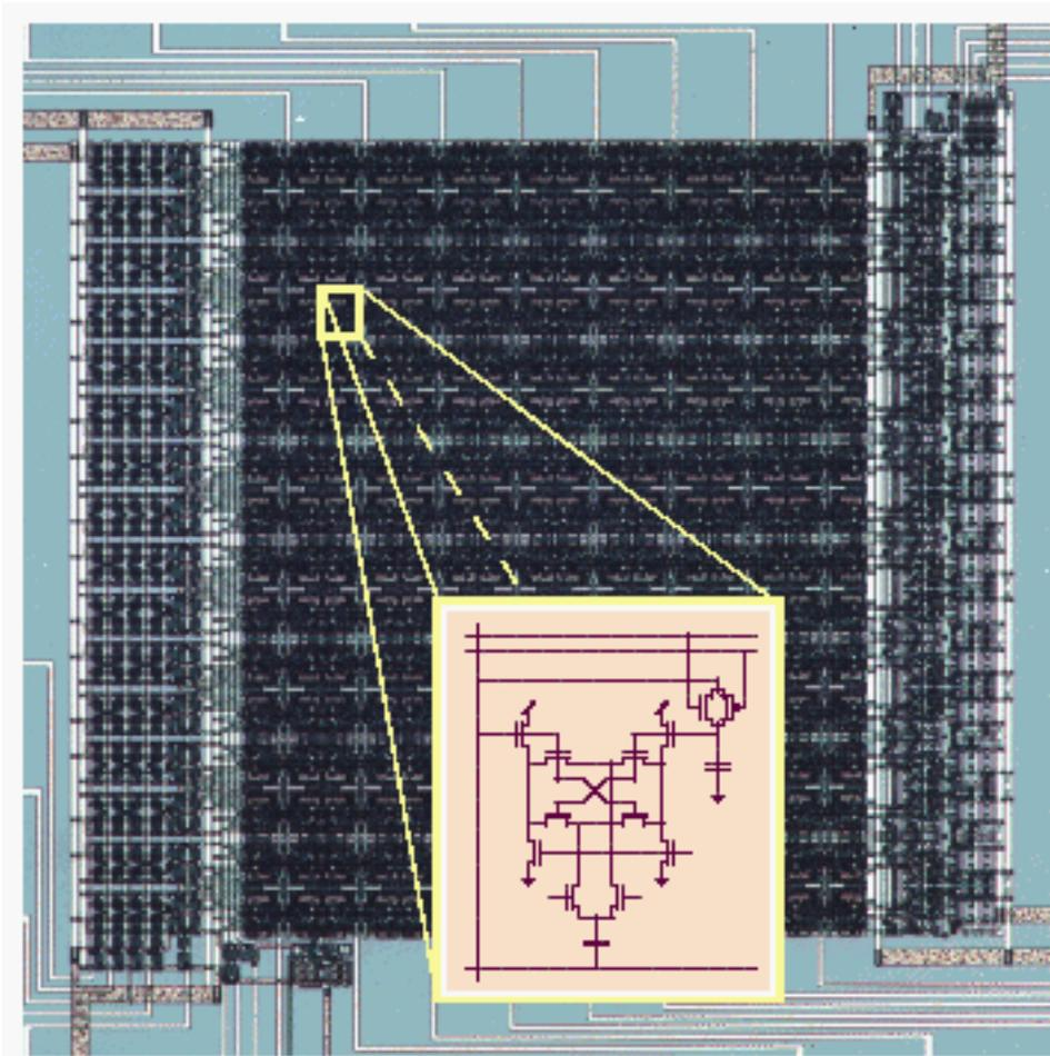
*Example: VLSI Analog-to-digital vector quantizer
