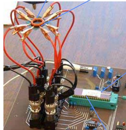
VLSI potentiostat array for distributed electrochemical sensing (Murari, Stanacevic, Cauwenberghs, and Thakor, 2004)
