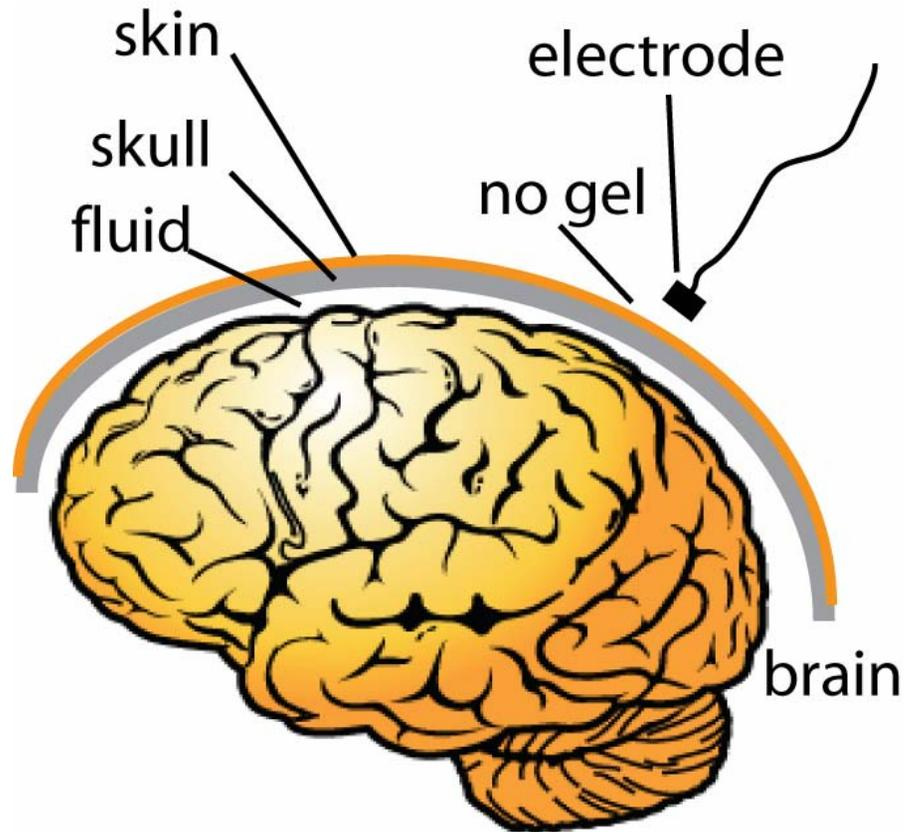
Capacitive coupling, rather than ohmic contact, between scalp/skin and electrode
