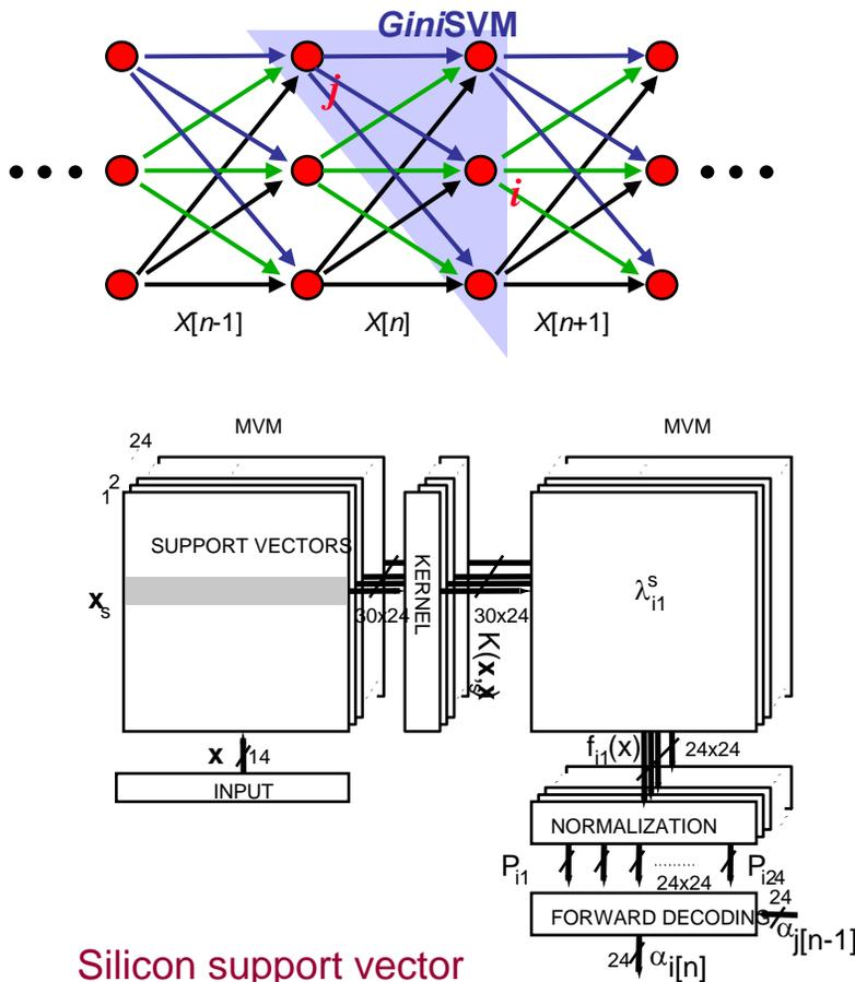
Silicon support vector machine (SVM) and forward decoding kernel machine (FDKM)
