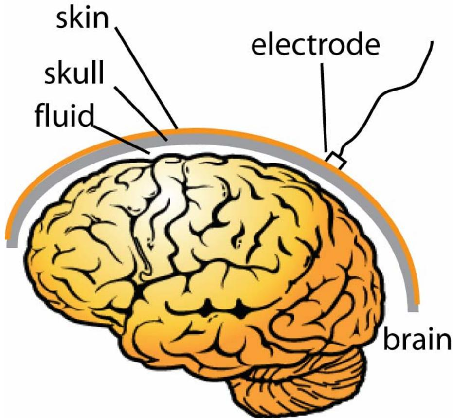
Dry-contact electrode penetrates outer layer of skin for ohmic contact without conductive gel.
