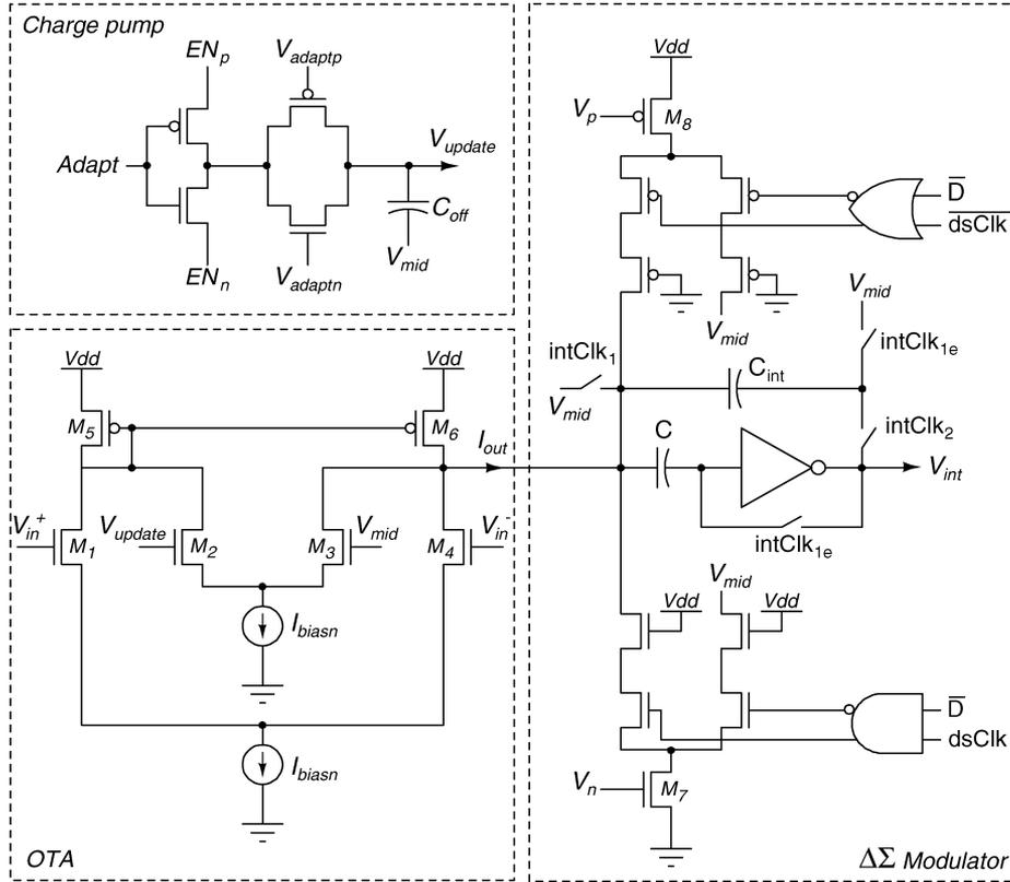
Fig. 3. Circuit schematic of the continuous-time Gm-C incremental  $\Delta\Sigma$  ADC, including adaptive offset cancellation.
