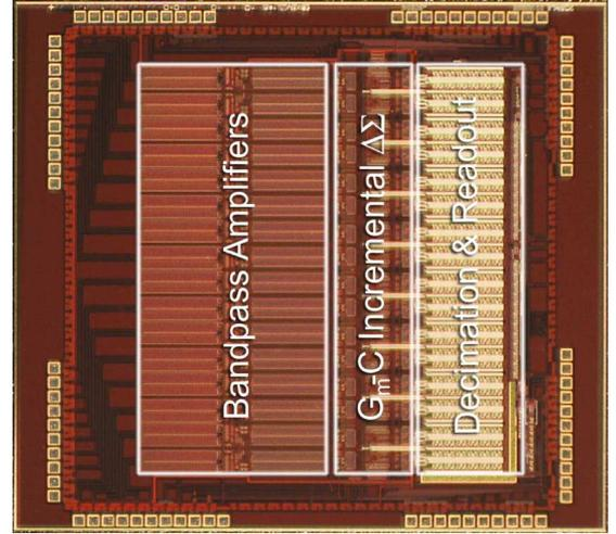
Fig. 4. Micrograph of the fabricated chip. Die size is  $3 \text{ mm} \times 3 \text{ mm}$  in  $0.5 \mu\text{m}$  3M2P CMOS technology.
