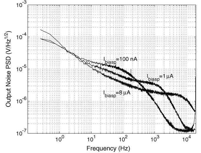
Fig. 6. Measured output noise density of the amplifier for different bias  $I_{\text{biasp}}$ .
