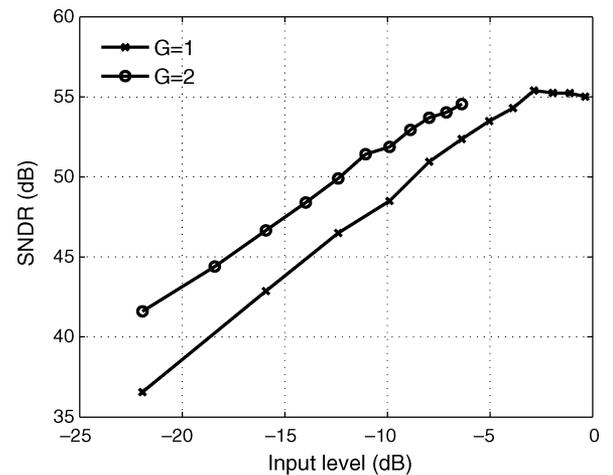
Fig. 8. Measured SNDR of the ADC for  $G = 1$ , and  $\text{OSR} = 10$ . Input level is relative to full scale ( $125 \text{ mV}_p$  sine wave input to the ADC).
