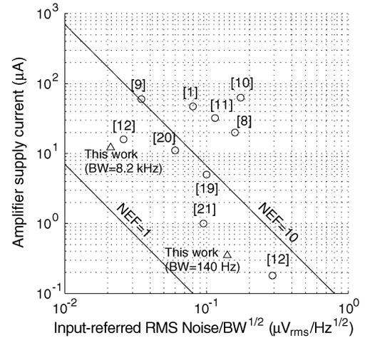
Fig. 7. Comparison of NEF between the presented amplifier (at two bandwidth settings, BW) and other designs in the literature.
