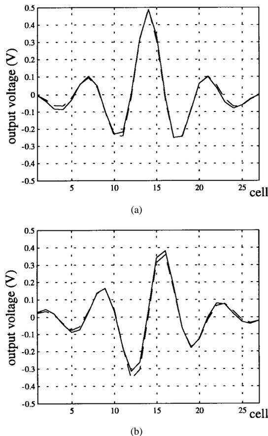
Fig. 6. Measured outputs from the array for  $\lambda/\alpha = 0.22$ . (a) The offset corrected even output (solid line) compared with the response of an ideal filter (dashed line). (b) The offset corrected odd output (solid line) compared with the response of an ideal filter (dashed line).
