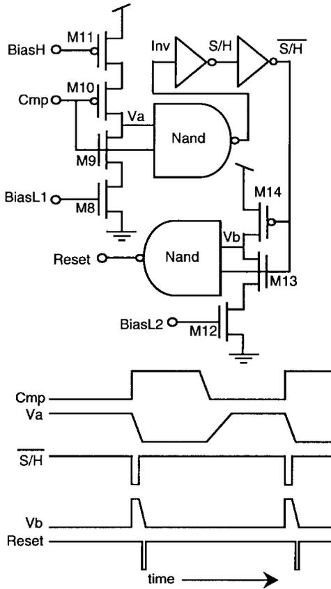
Fig. 4. Control pulse generator: The bias voltage  $Bias_H$  controls the rising slope and  $Bias_{L1}$ ,  $Bias_{L2}$  control the falling slope, thus, creating a time delay element.
