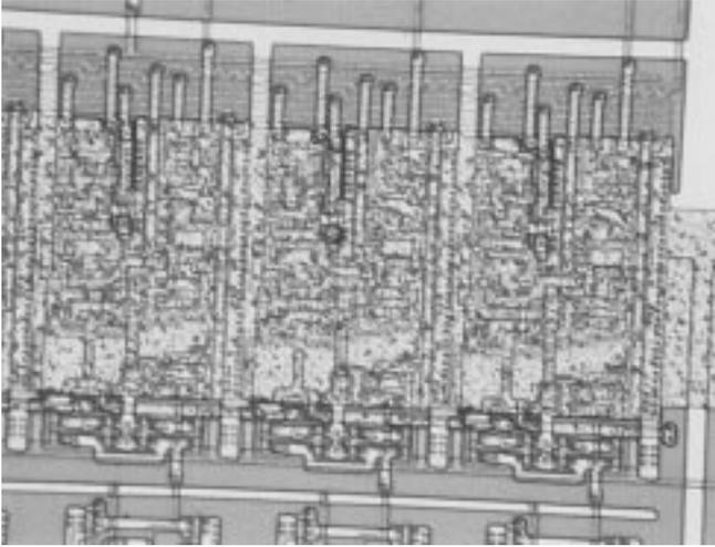
Fig. 5. Photomicrograph of three zero crossing cells on the chip. The cell dimension is  $120 \mu\text{m} \times 227 \mu\text{m}$  each, fabricated in N-well  $2\text{-}\mu\text{m}$  CMOS technology.
