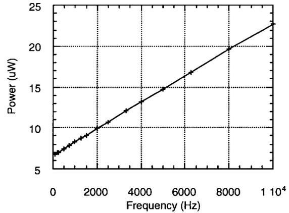
Fig. 9. Power consumption of the fabricated cell with a 5-V power supply.
