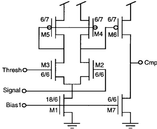
Fig. 3. Comparator circuit: A two-stage amplifier operated in an open loop configuration.
