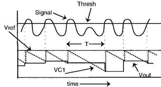
Fig. 2. Block diagram for a single cell: time intervals are computed by integrating a constant current on a capacitor.
