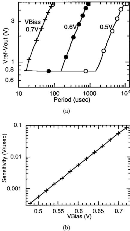
Fig. 7. (a) Output voltage versus input signal period, at three different discharge current bias settings and (b) output sensitivity versus bias voltage.
