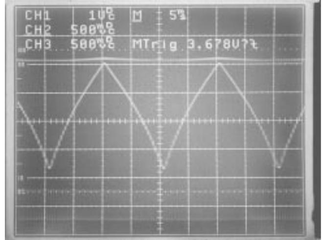
Fig. 6. Output waveform for a frequency modulated input—The lower waveform is the frequency modulated input, upper waveform (the straight line and thin vertical lines) show the resetting and discharging of the capacitor, and the triangular wave is the final output.
