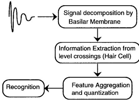
Fig. 1. Neuromorphic architecture for sensory preprocessing. Unlike the more traditional approach, the quantization of signal occurs at a much higher level and thus a single chip preprocessor replaces functions traditionally performed by the A/D converters and specialized digital signal microprocessors (DSP chips).
