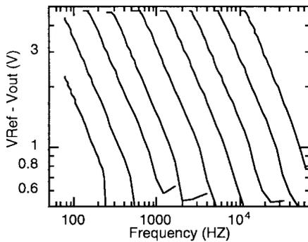
Fig. 8. Frequency-to-voltage characteristics of the transducer array over the audio frequency range.
