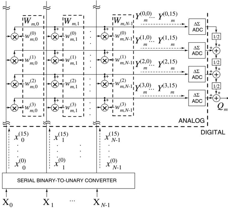
Fig. 5. Block diagram of one row of the matrix with binary encoded elements  $w^{(i)}_{mn}$ , for a single  $m$  and  $I = 4$ . Data flow of bit-serial unary encoded inputs  $x^{(j)}_n$  and corresponding partial product outputs  $Y^{(i,j)}_m$ , with  $J = 16$  bits. The full product for a single row  $Y^{(i)}_m$  is accumulated and quantized by a delta-sigma ADC. The final product is constructed in the digital domain according to 18.
