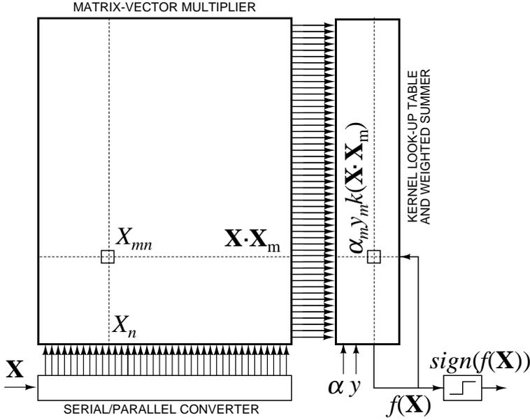
Fig. 3. The architecture of the core recognition processor for support vector machine classification and on-line training. Communication with outside modules is through a serial digital input/output interface for maximal flexibility and programmability, while the core internal computations are parallel and analog for optimal efficiency.
