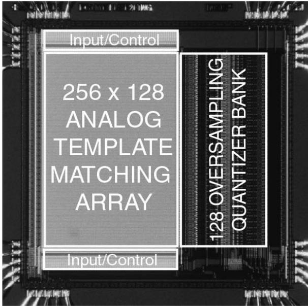
Fig. 4. Micrograph of the *Kerneltron* prototype, containing an array of  $256 \times 128$  computational cells with embedded memory, and a row-parallel bank of 128 algorithmic  $\Delta\Sigma$  ADCs. Die size is  $3 \text{ mm} \times 3 \text{ mm}$  in  $0.5 \mu\text{m}$  CMOS technology.
