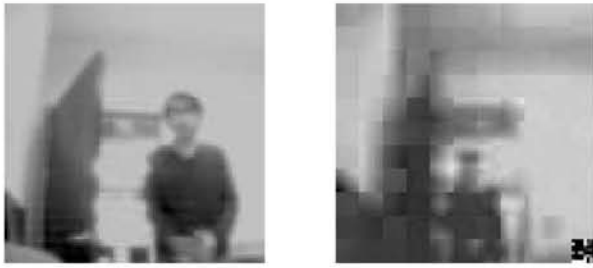
Fig. 4. Video output from sensor board at 50:1 (right) and 5:1 (left) compression rates.
