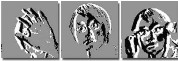
Fig. 1. Imager change detection output [8] showing a person moving in the frame. Positive change threshold events are shown in white, and negative change threshold events are shown in black. Change events of either polarity trigger DCT encoding and transmission of imager intensity output over an 8x8 block of pixels.
