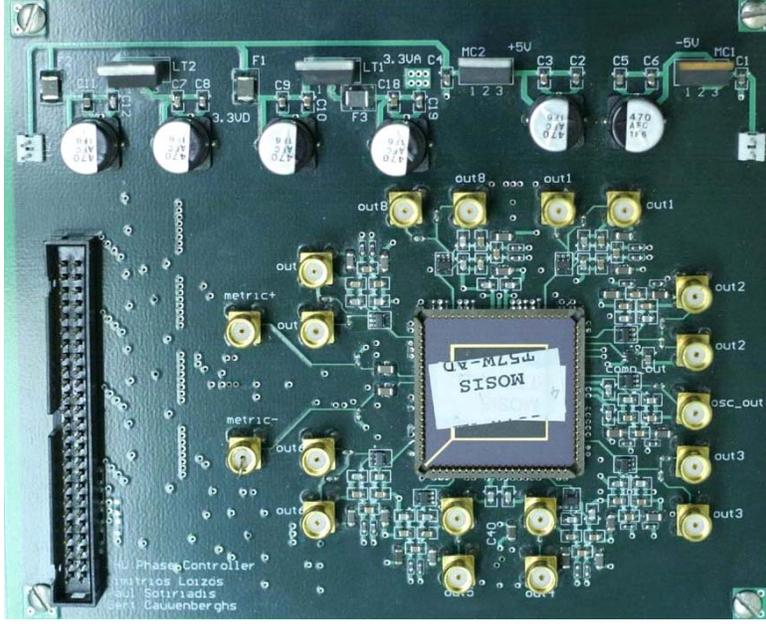
Figure 3: VLSI multi-dithering controller developed at the Johns Hopkins University (2006). Dither frequency range: 100Hz~800MHz. Channel output dynamic range: 0.5~2.5V. The IDC50 connector is for interfacing to PC card (PCI-DAC6703). Power supplies are 0.0~+3.0V. There are eight output channels and each channel has two output terminals with 50Ω output impedance. There are two differential metric inputs terminals with 50Ω input impedance.
