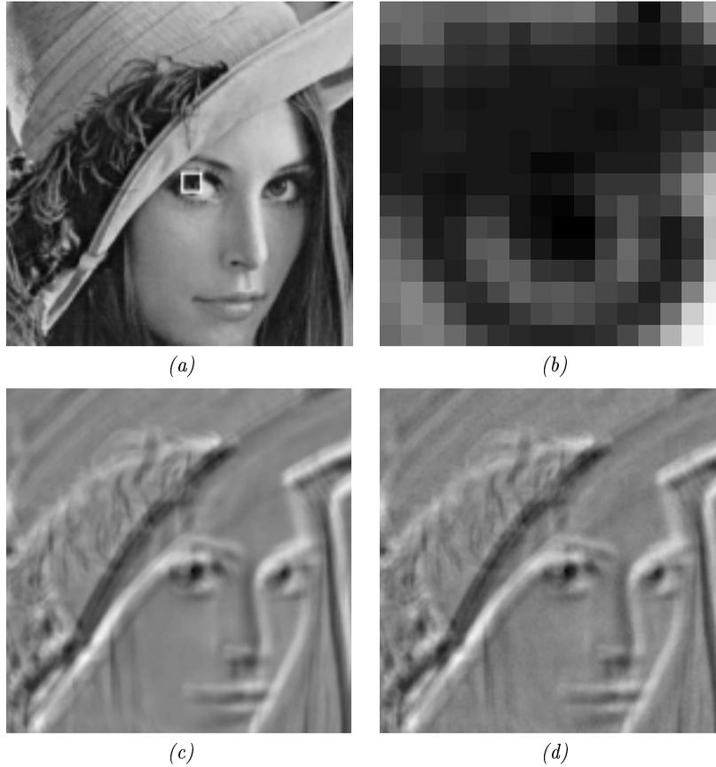
**Fig. 6.** Cross-correlation of fragments of *Lena* (a) and the eye template (b) computed by a 32-bit floating point processor with 8-bit encoded inputs (c) and by *Kerneltron* with 8-bit quantization and 4-bit encoded inputs (d).
