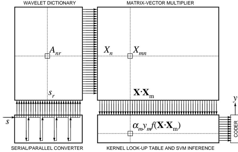
**Fig. 2.** The architecture of the core recognition processor, combining overcomplete wavelet decomposition with generalized support vector machine classification. Communication with outside modules is through a serial digital input/output interface for maximal flexibility and programmability, while the core internal computations are parallel and analog for optimal efficiency.
