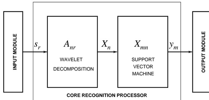
**Fig. 1.** Functional block diagram of the SVM classifier. The core of the system is a support vector machine processor for general object detection and classification. An overcomplete wavelet decomposition of the incoming sensory data at the input generates redundant input features to the SVM, providing for robust and relatively invariant classification performance.
