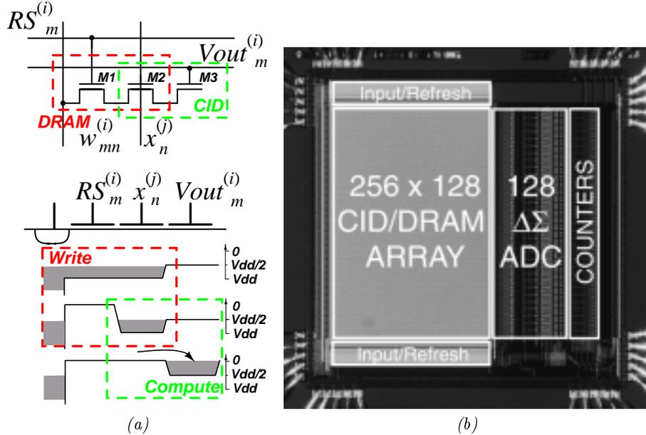
**Fig. 3.** (a) CID computational cell with integrated DRAM storage. Circuit diagram, and charge transfer diagram for active write and compute operations. (b) Micrograph of the *Kerneltron* prototype, containing containing an array of  $256 \times 128$  CID/DRAM cells, and a row-parallel bank of 128 algorithmic  $\Delta\Sigma$  ADCs. Die size is  $3 \text{ mm} \times 3 \text{ mm}$  in  $0.5 \mu\text{m}$  CMOS technology.
