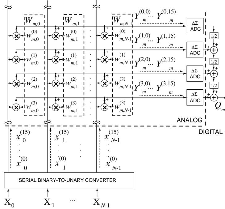
**Fig. 5.** Block diagram of one row of the matrix with binary encoded elements  $w_{mn}^{(i)}$ , for a single  $m$  and  $I = 4$ . Data flow of bit-serial unary encoded inputs  $x_n^{(j)}$  and corresponding partial product outputs  $Y_m^{(i,j)}$ , with  $J = 16$  bits. The full product for a single row  $Y_m^{(i)}$  is accumulated and quantized by a delta-sigma ADC. The final product is constructed in the digital domain according to (10).
