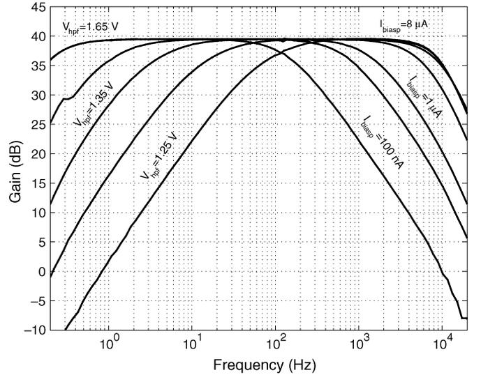
Fig. 5. Filter response for lowpass current bias  $I_{\text{biasp}}$  between 100 nA and 8  $\mu\text{A}$ , and for highpass voltage bias  $V_{\text{hpf}}$  between 1.25 and 1.65 V.
