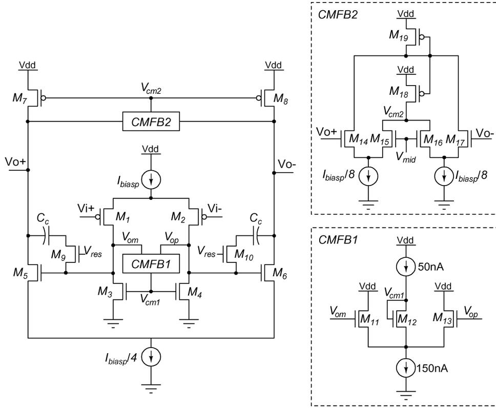
Fig. 2. Fully differential two-stage amplifier in the bandpass amplifier frontend of Fig. 1.
