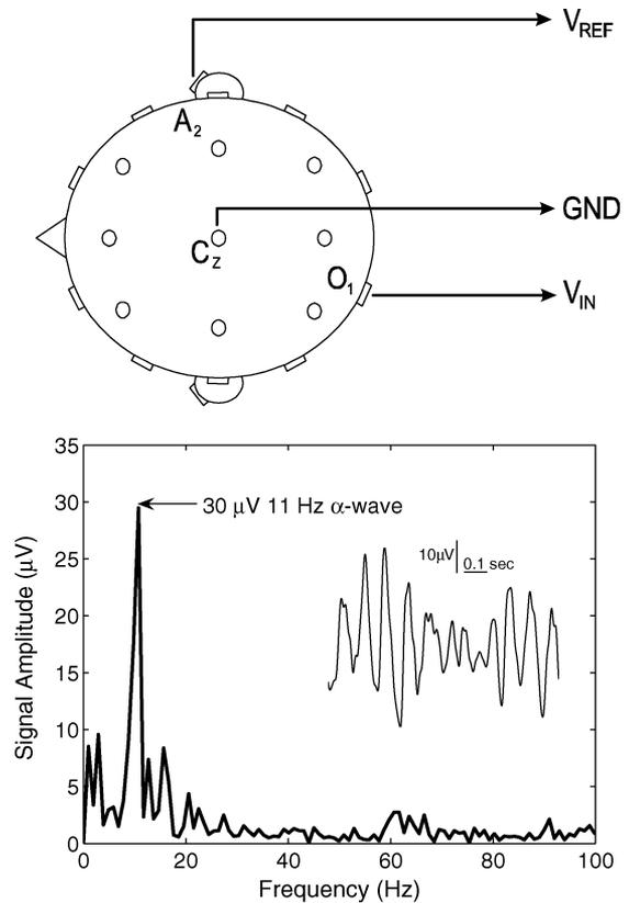
Fig. 11. Experimental setup for EEG recording and recorded waveform from occipital lobe, with the subject's eyes closed, showing alpha wave activity.
