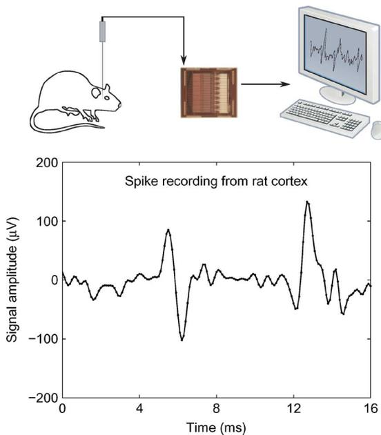
Fig. 10. *In-vivo* neural signal recording. Spikes were recorded from rat somatosensory cortex using a tungsten electrode. A screw electrode was used as signal ground.
