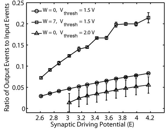
Fig. 8. Average ratio of output events to input events versus synaptic reversal potential  $E$ , measured in volts. Data are averaged across ten trials per cell at each value of synaptic weight, and then averaged across all 2400 cells. Error bars represent  $\pm 1$  standard deviation.
