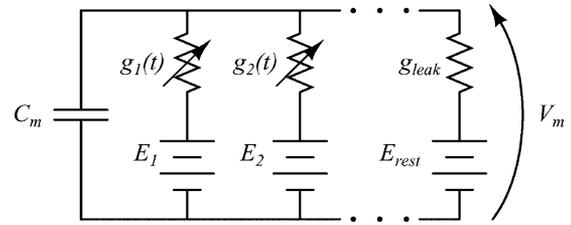
Fig. 3. Single-compartment model of a biological neuron with transmembrane voltage  $V_m$ , lumped membrane capacitance  $C_m$ , multiple synapses represented by  $\{g_i(t), E_i\}$  pairs, and a static leak conductance to the resting potential  $\{g_{\text{leak}}, E_{\text{rest}}\}$ .
