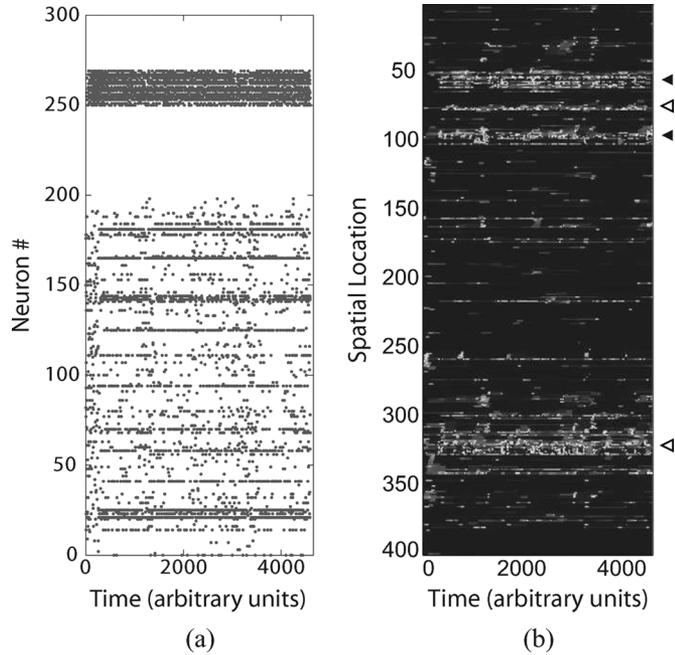
Fig. 13. Example of partial remapping and stable activity bumps. (a) IFAT output events from excitatory neurons 0–199 and inhibitory neurons 250–269 plotted as neuron number versus time. (b) IFAT output events plotted as spatial location versus time. Color scale as in Fig. 12. Arrowheads point to activity bumps; see text for details.
