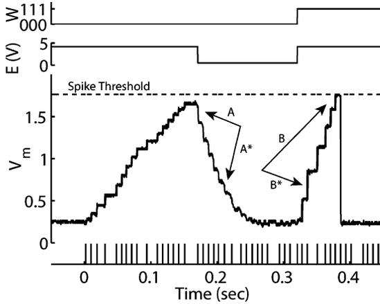
Fig. 6. Data captured from an oscilloscope during operation of the chip. The lower trace illustrates the membrane potential ( $V_m$ ) of a single neuron in the array as a series of events are sent at times marked by vertical lines at the bottom of the figure. The synaptic reversal potential ( $E$ ) and synaptic weight ( $W$ ) are drawn in the top two traces. Arrow labeled  $A$  points to the effects of a “shunting” inhibitory input. See text for description of other symbols.
